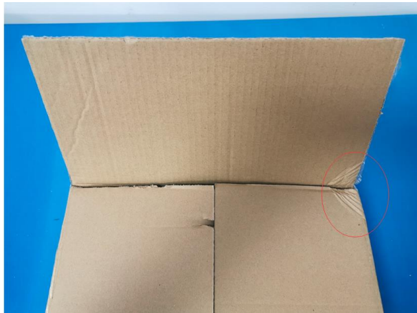
Crushed corner and edge
